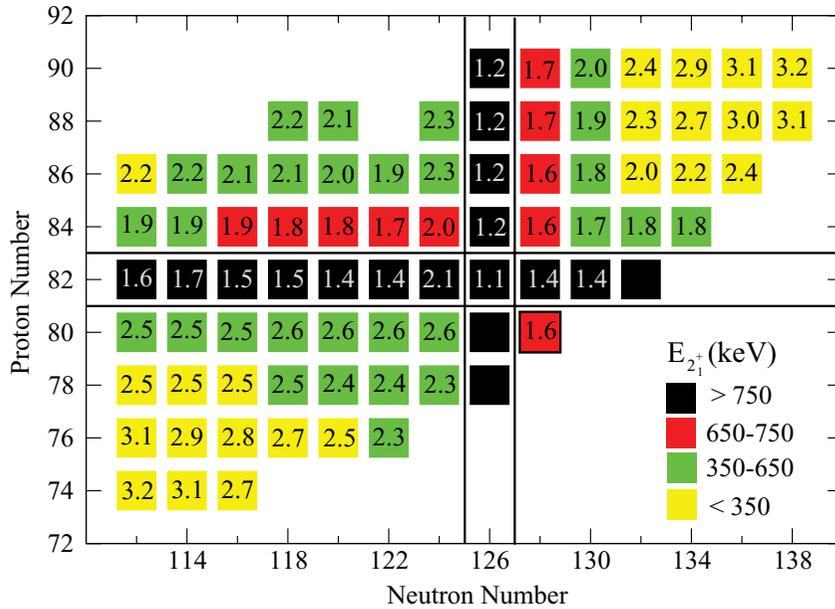
FIG. 3. (Color online) Systematics of the  $E(2^+)$  energies and the  $E(4^+)/E(2^+)$  energy ratios for even-even nuclei around  $^{208}\text{Pb}$ . The red box with a black square is from the current work on  $^{208}\text{Hg}$ .
