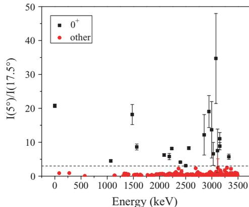
FIG. 2. (Color online) Measured ratio of the cross sections at  $5^\circ$  and  $17.5^\circ$ . The dashed line gives the limit above which levels are assigned to be  $0^+$  states.
