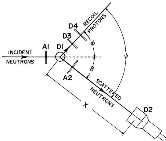
FIG. 3. A schematic diagram of the time-of-flight spectrometer.
