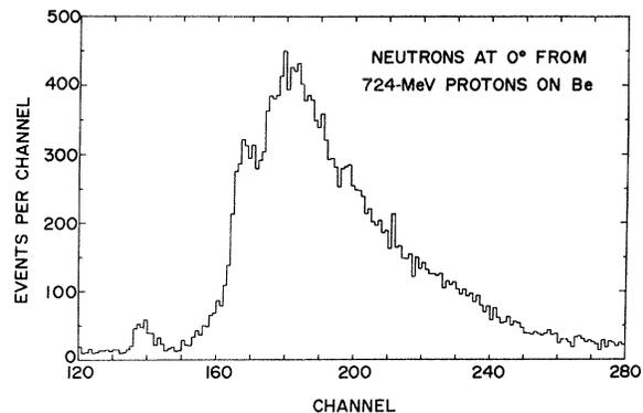
FIG. 4. Neutron time-of-flight spectrum at  $0^\circ$  from 724-MeV proton bombardment of beryllium. This measurement was made with an NE-228 liquid D1 scintillator.
