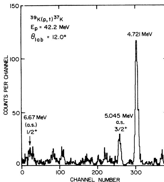
FIG. 2. A portion of the  $^{39}\text{K}(p, t)^{37}\text{K}$  spectrum at  $E_p = 42.2$  MeV and  $\theta = 12^\circ$ .
