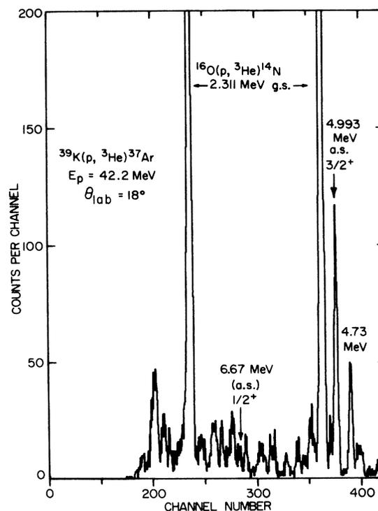
FIG. 4. A portion of the  $^{39}\text{K}(p, ^3\text{He})^{37}\text{Ar}$  spectrum at  $E_p = 42.2$  MeV and  $\theta = 18^\circ$ .
