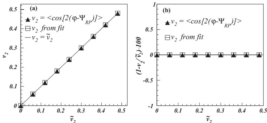
FIG. 4. (a)  $v_2$  extracted from generated azimuthal distributions as a function of input  $\tilde{v}_2$  in the case of anisotropy applied via Eq. (8). (b) Relative difference between resulting  $v_2$  and input  $\tilde{v}_2$ .
