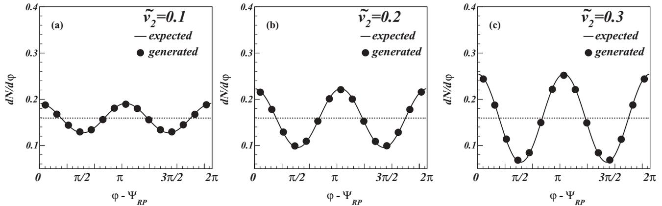
FIG. 3. Azimuthal distributions of particles generated isotropically and transformed with Eq. (8) for three values of input  $\tilde{v}_2$ . The expected  $1 + 2\tilde{v}_2 \cos[2(\varphi - \Psi_{RP})]$  trend is superimposed. The dotted line indicates azimuthal isotropic distribution of the particles ( $dN/d\varphi = 1/2\pi$ ).
