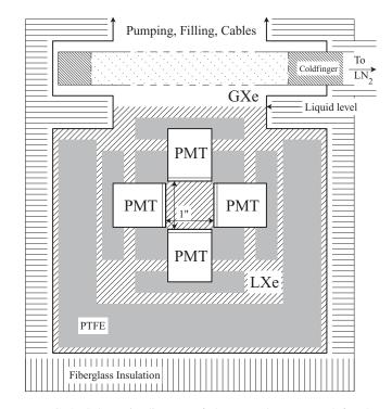
FIG. 2. Schematic diagram of the LXe detector used for the  $\mathcal{L}_{\text{eff}}$  measurement. Visible are four of the six PMTs used to view the 1-in.<sup>3</sup> active LXe volume.
