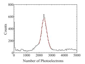
FIG. 3. (Color online) The scintillation light spectrum of 122-keV  $\gamma$  rays from <sup>57</sup>Co, used to calibrate the electronic recoil energy scale. This calibration gives a scintillation yield of 19.64 p.e./keV.
