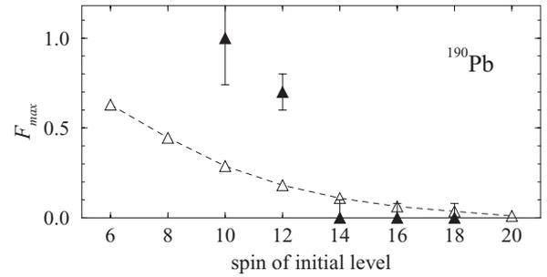
FIG. 7.  $F_{\max}$  estimated for  $^{190}\text{Pb}$  (open symbols) assuming that the SD band in this nucleus is 0.5 MeV closer to the yrast line than the band in  $^{192}\text{Pb}$ , and experimental fractional intensity loss profile (close symbols) for this nucleus.
