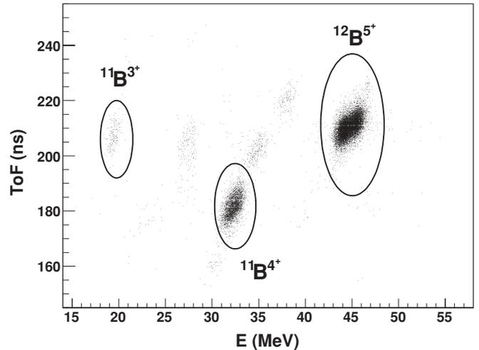
FIG. 2. Composition of the secondary  $^{12}\text{B}$  beam obtained with a Si  $\Delta E$ - $E$  detectors at the secondary target position. The start signal for the TOF measurements was taken from the E detector, and the stop signal came from the RF of the buncher (reverse TOF). The  $^{11}\text{B}^{3+}$  ions are from the preceding (with respect to  $^{12}\text{B}$ ) bunch.
