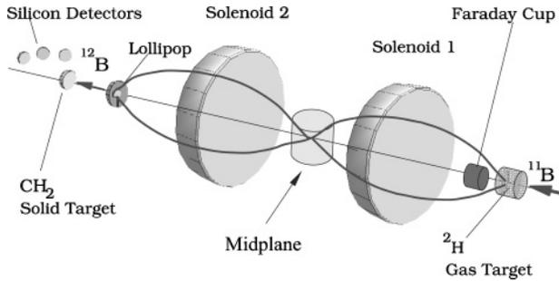
FIG. 1. The experimental setup with beam trajectories through TwinSol. The “lollipop” reduces contamination of the beam by intercepting ions that focus at a different location relative to  $^{12}\text{B}$ .
