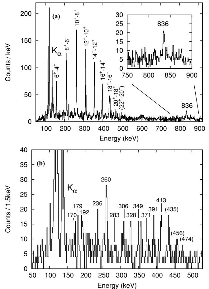
FIG. 2. (a) Spectrum of  $\gamma$  rays detected in the JUROGAM array when a fusion-evaporation residue is observed at the focal plane of RITU. (b) As in (a), with the additional requirement that an electron sum event is observed within 10 s of the recoil at the same position in the DSSD.
