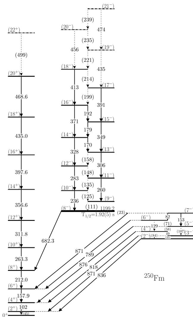
FIG. 3. Partial level scheme of  $^{250}\text{Fm}$  deduced in the present work. The ground state rotational band had previously been observed up to a spin of  $18\hbar$  [5]. The  $M1$  transition energies in the  $K^\pi = 8^-$  band are marked for clarity though a large number of them were not observed. The error on the transition energies shown is  $\pm 0.5$  keV for those marked to one decimal place and  $\pm 1$  keV for those marked with integer numbers.
