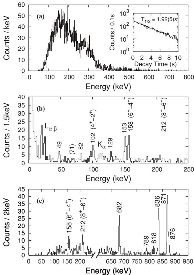
FIG. 1. (a) Spectrum of “sum energy” electrons observed within 10 s of a fusion-evaporation residue at the same position in the DSSD. (b) Gamma rays detected in prompt coincidence with the electrons of part (a) in the planar germanium detector. (c) As in (b), but in the array of clover detectors.
