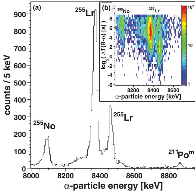
FIG. 1. (Color online) (a) Total  $\alpha$ -particle energy spectrum measured at the focal plane. (b) A logarithmic plot of the time difference between position-correlated  $\alpha$ -particles and recoils as a function of  $\alpha$ -particle energy.
