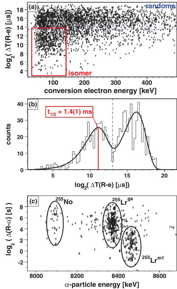
FIG. 2. (Color online) (a) A logarithmic plot of the time difference between recoil and conversion electron detection ( $\log_2(\Delta T(R-e))$ ) as a function of conversion electron energy. (b) Time differences for conversion electrons with energies less than 140-keV [projection of (a) onto the y-axis]. (c) Decay time as a function of energy for position correlated  $\alpha$  particles in coincidence with the isomeric conversion electron decay.
