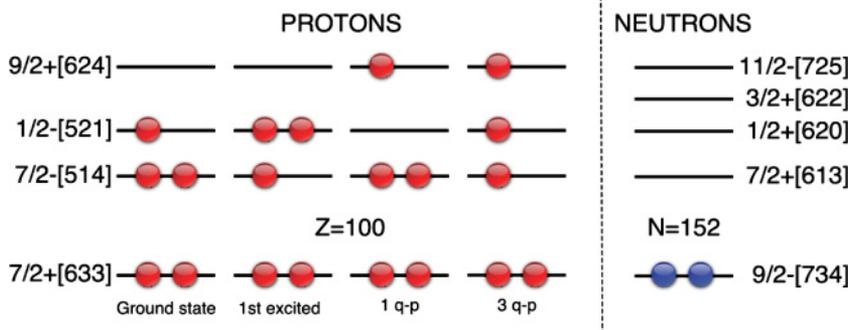
FIG. 5. (Color online) Schematic representation of the available proton (left) and neutron (right) configurations based on the single-particle levels calculated in Ref. [22].
