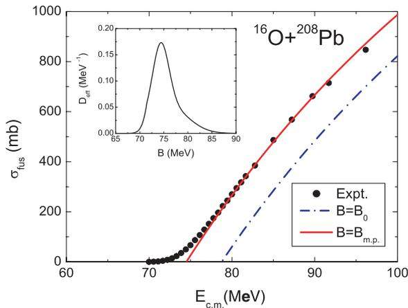
FIG. 2. (Color online) Fusion excitation function of the reaction  $^{16}\text{O} + ^{208}\text{Pb}$ . The dash-dotted and solid curves denote the calculated results with Eq. (5) by taking  $B = B_0$  and  $B = B_{m.p.}$ , respectively. The solid circles denote the experimental data [27]. The inset shows the effective weight function of the reaction.
