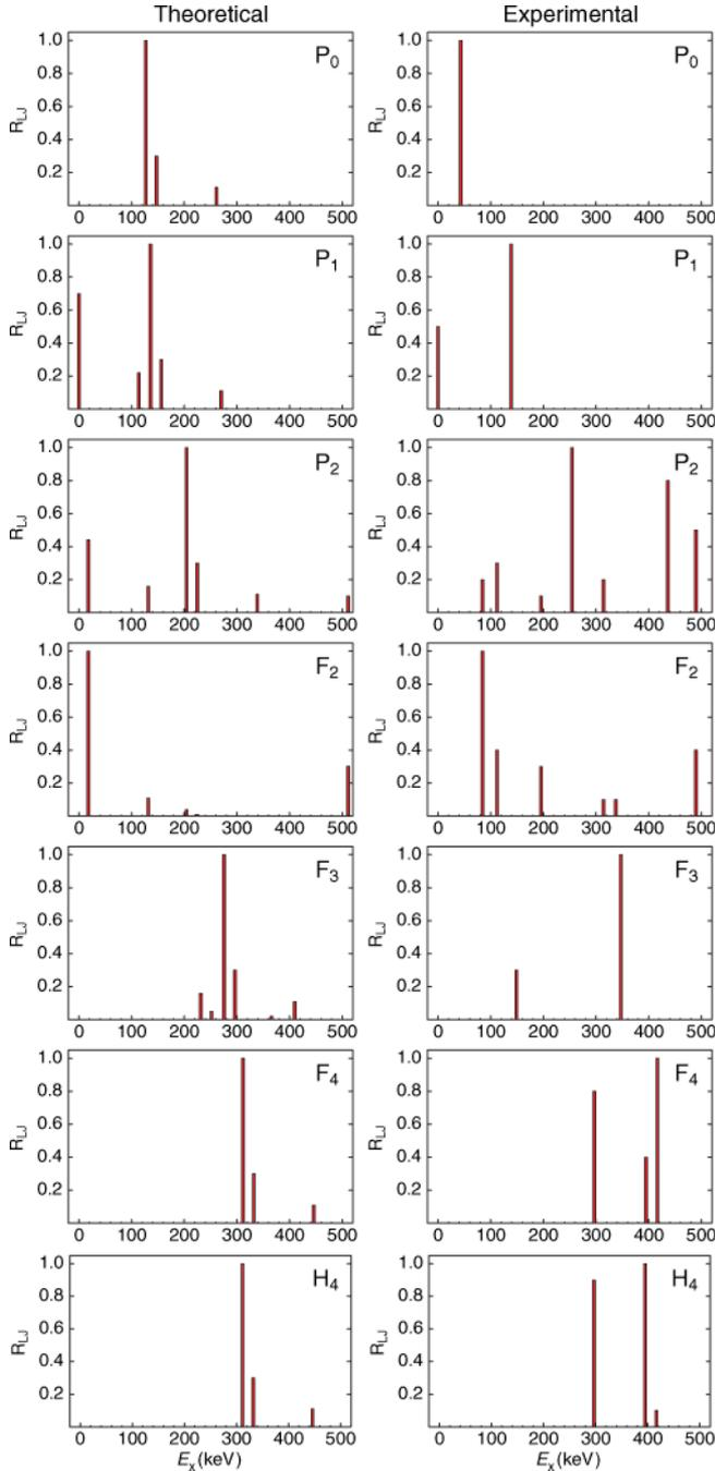
FIG. 5. (Color online) Comparison of theoretical and experimental values of ratios  $R_{LJ}$  of spectroscopic strengths (cf. Table VIII).
