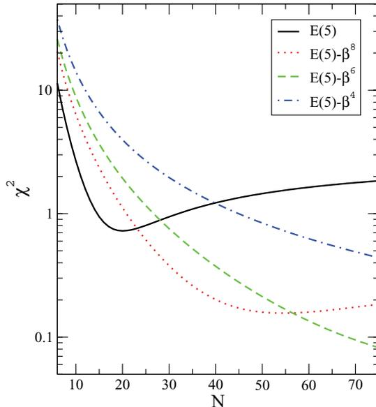
FIG. 4. (Color online)  $\chi^2$  values for the  $E2$  transition rates for the different E(5) models, as a function of  $N$ , and an IBM electromagnetic operator  $T(E2) = e_{\text{eff}}(s^\dagger \bar{d} + d^\dagger \bar{s})$ .
