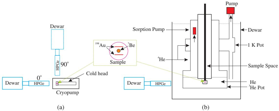
FIG. 1. (Color online) (a) Schematics of the setup for the measurements at 12.5 K and 293 K (“experiment 1”) at the  $0^\circ$  and  $90^\circ$  geometry assemblies. (b) Schematics of the setup for the measurement at 0.350 K and 4 K (“experiment 2”) at the  $90^\circ$  geometry assembly.
