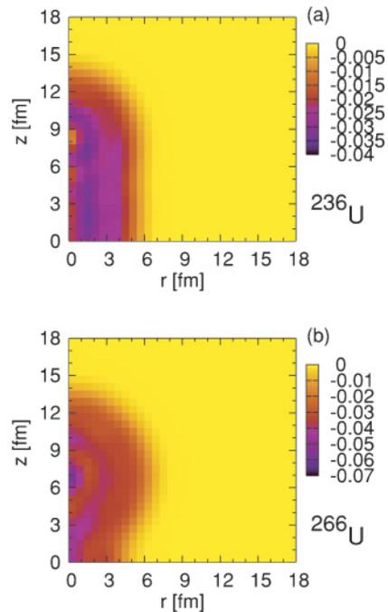
FIG. 7. (Color online) Difference of the proton and the neutron density distributions,  $\rho_p - \rho_n$ , for  $^{236}\text{U}$  (Fig. 7(a)) and  $^{266}\text{U}$  (Fig. 7(b)) at  $\beta_t = 2.0$  obtained with the total constraint. The densities are axial symmetric around the  $z$ -axis.
