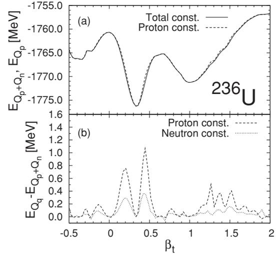
FIG. 3. The fission barrier for  $^{236}\text{U}$  as a function of deformation parameter  $\beta_t$  obtained with the total constraint scheme (Fig. 3(a)). The dashed line in the Fig. 3(b) shows the difference of the fission barrier obtained with the proton constraint and that with the total constraint, while the dotted line denotes the difference obtained with the neutron constraint.
