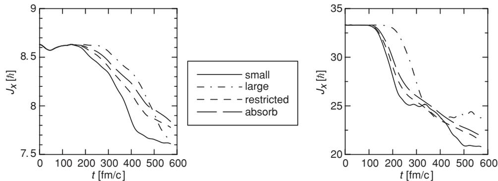
FIG. 3. Angular momentum as a function of time for collisions of  $^{16}\text{O}+^{16}\text{O}$  at  $E_{\text{c.m.}} = 25$  MeV (left) and 125 MeV (right). The different cases are: “small”: calculation in a grid of  $24 \times 32 \times 32 \text{ fm}^3$ , “large”: calculation in a grid doubled in total size in every direction, “restricted”: same as large, but angular momentum is summed up only over the small grid; “absorb”: small grid with a 6 fm absorbing layer around the boundary.
