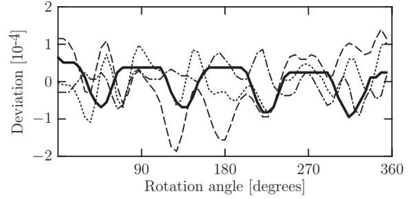
FIG. 2. Relative deviations of the angular momentum expectation value (full curve) and the three principal moments of inertia (smallest: dotted, intermediate: dashed, and largest: dot-dashed curve) from the temporal average during rotation of a  $^{24}\text{Mg}$  nucleus. The abscissa denotes the rotation angle calculated from the instantaneous tensor of inertia.
