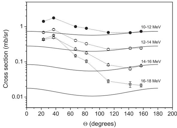
FIG. 1. Angular distributions of  $\alpha$  particles in the c.m. system for different energy intervals. The points are experimental data and the solid lines are HF calculations normalized to match the experimental points at backward angles for low energy particles.
