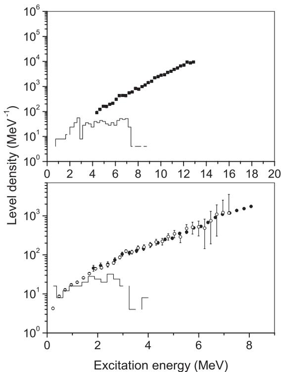
FIG. 4. Level densities of  $^{47}\text{Ti}$  (upper panel) and  $^{44}\text{Sc}$  (lower panel) nuclei obtained from proton and  $\alpha$ -particle energy spectra, respectively. Black points are data from particle evaporation spectra. Open points are data from the Oslo experiment [7]. The histograms represent level densities from the counting of discrete levels.
