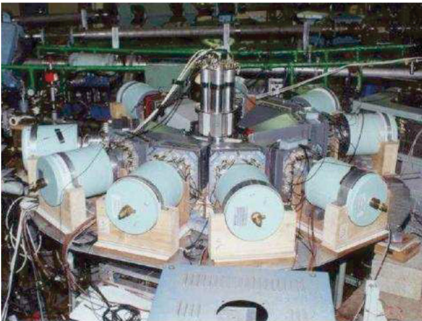
FIG. 1. (Color online) INGA setup comprising of eight Clover detectors at TIFR.
