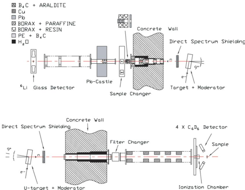
FIG. 1. (Color online) Experimental arrangement for the transmission (above) and the capture (below) measurements performed at the GELINA neutron time-of-flight facility.
