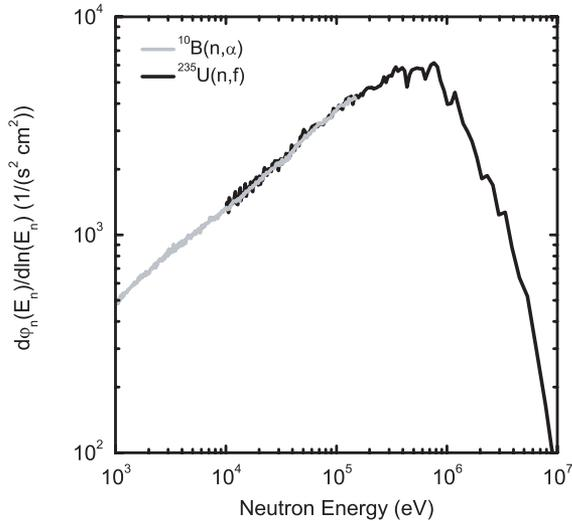
FIG. 2. The neutron spectrum at the 58-m capture station, obtained from  $^{10}\text{B}(n, \alpha)$  and  $^{235}\text{U}(n, f)$  measurements, with the accelerator operating at 800 Hz.
