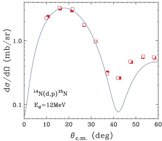
FIG. 1. (Color online) Comparison of tabulated data (closed points) [25] and digitized data (open points) [86] from the same measurement of the angular distributions of the protons obtained in the  $^{14}\text{N}(d, p)^{15}\text{N}$  reaction at incident deuteron energy of 12 MeV. The curve is the predicted angular distributions from the code TWOFNR as described in the text, multiplied by 1.1, which is the spectroscopic factor.
