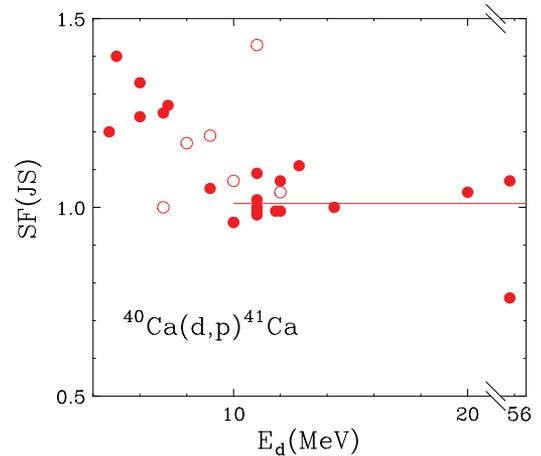
FIG. 5. (Color online) Comparison of spectroscopic factors, SF(JS), obtained from Ref. [186] (open circles) and from other measurements (closed circles). The increase of spectroscopic factors observed at  $E_d < 10$  MeV has been observed before [22,25] and attributed to the resonance structures in the elastic scattering of the deuterons [253]. Solid line is the mean SF(JS) between 10 and 56 MeV.
