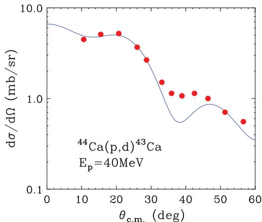
FIG. 2. (Color online) Angular distributions of the deuteron obtained in the  $^{44}\text{Ca}(p, d)^{43}\text{Ca}$  reaction at incident proton energy of 40 MeV [179]. The curve is the predicted angular distributions from the code TWOFNR as described in the text, multiplied by the spectroscopic factor.
