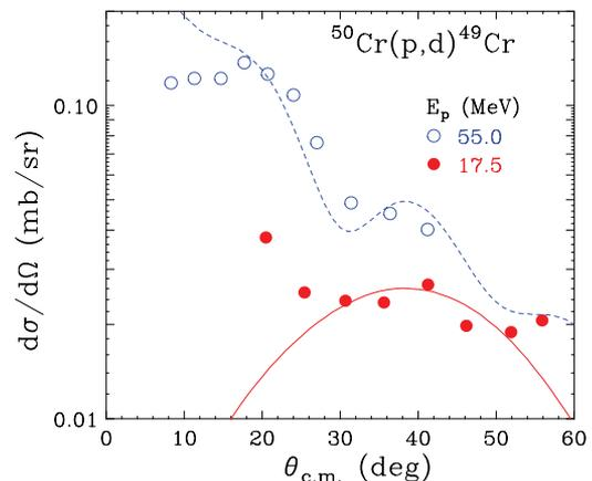
FIG. 7. (Color online) Comparison of angular distributions of the deuteron measured in the  $^{50}\text{Cr}(p,d)^{49}\text{Cr}$  reactions in two different experiments: Ref. [229] (closed circles) and Ref. [230] (open circles).
