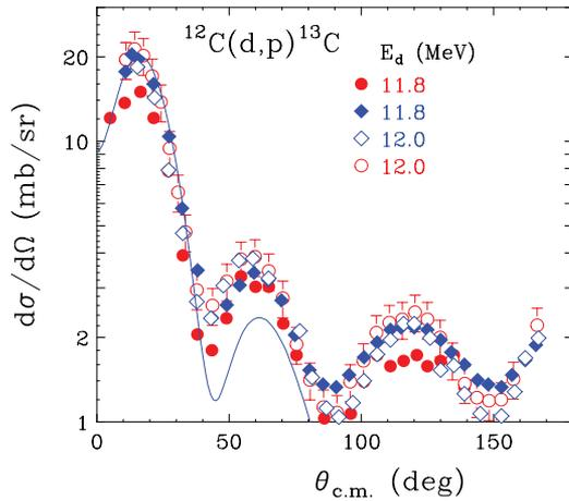
FIG. 4. (Color online) Comparison of the angular distributions of the proton measured in the  $^{12}\text{C}(d,p)^{13}\text{C}$  reactions in four different experiments: Ref. [25] (open circles), Ref. [49] (closed circles), Ref. [63] (open diamonds), and Ref. [34] (closed diamonds). The curve is the predicted angular distributions from the code TWOFNR multiplied by the spectroscopic factor.
