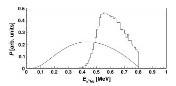
FIG. 8.  $E_{\alpha^{5}\text{He}}$  profile deduced from calculation (solid curve) and from simulation (histogram) assuming a  $W(\theta)$  function defined by the parameters  $A_0 = 0.737$  and  $A_2 = -0.526$ . The distribution obtained from simulation is normalized to the calculation for comparison.
