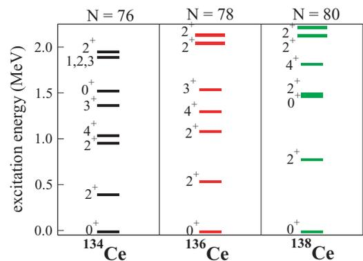
FIG. 6. (Color online) Comparison of energy levels in Ce isotopes. The larger lines represent the candidates for the fragmented  $2_{1,ms}^+$  state in  $^{136}\text{Ce}$  and the fragmented  $2_{1,ms}^+$  state in  $^{138}\text{Ce}$ .
