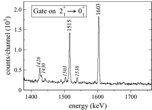
FIG. 2. The  $\gamma$ -ray spectrum observed from the  $^{136}\text{Pr}$   $\beta$  decay. Displayed is one energy region of interest in the coincidence spectrum gated on the 552-keV ( $2_1^+ \rightarrow 0_1^+$ ) transition for Ge detectors at a relative angle of  $90^\circ$  (Group 1).
