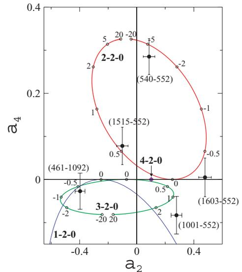
FIG. 5. (Color online) The theoretical ellipses for the  $a_2$  and  $a_4$  angular correlation coefficients plotted parametrically as functions of  $\delta_1$  for quadrupole-dipole mixing are shown along with the data (filled circles) for the (552–540)-, (552–1515)-, (552–1603)-, (461–1092)-, and (1001–552)-keV cascades. Values of  $\delta_1$  on the ellipses are denoted with open circles.
