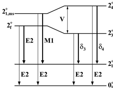
FIG. 8. Schematic of a two-state mixing scenario for the  $2_{1,\text{ms}}^+$  mixed-symmetry state and a  $2_f^+$  fully-symmetric state.
