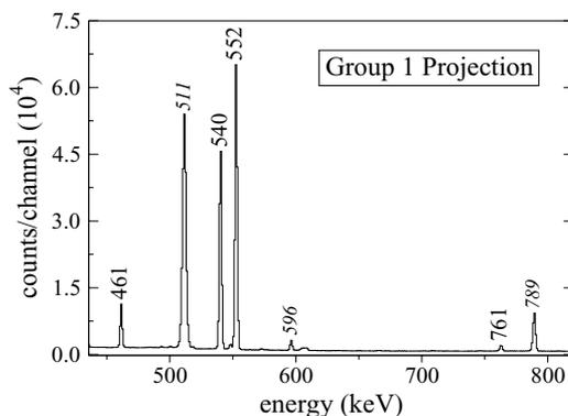
FIG. 1. The  $\gamma$ -ray spectrum observed from the  $^{136}\text{Pr}$   $\beta$  decay. Displayed is the lower energy portion of the  $\gamma\gamma$  coincidence matrix projection observed with Ge detectors at a relative angle of  $90^\circ$  (Group 1).
