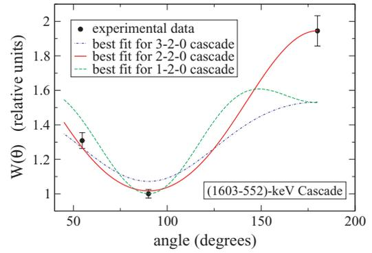
FIG. 4. (Color online) Angular correlation functions fitted to data for 3-2-0, 2-2-0, and 1-2-0 spin hypotheses with the  $E2/M1$  multipole mixing ratio for the preceding transition,  $\delta_1$ , treated as a free parameter in each case.
