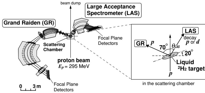
FIG. 1. Overview of the two-arm magnetic spectrometer system, consisting of Grand Raiden (GR) and the Large Acceptance Spectrometer (LAS).
