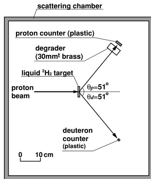
FIG. 2. Schematic view of the luminosity monitor (side view). Two plastic scintillation counters were placed at 51 degrees and at 20 cm from the target. A degrader made of brass with a thickness of 30 mm was used for stopping deuterons from entering the proton counter.
