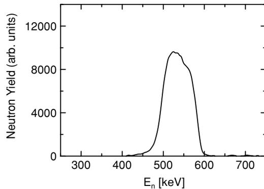
FIG. 1. Neutron energy spectrum taken by a  ${}^6\text{Li}$  glass scintillation detector with a TOF method.
