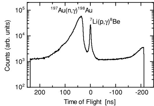
FIG. 2. TOF spectrum for  ${}^{197}\text{Au}$  taken by the NaI(Tl) detector at  $E_n = 531$  keV. The peak at 0 ns is from the  ${}^7\text{Li}(p, \gamma){}^8\text{Be}$  reaction and the broad peak is due to the  $\gamma$  ray from the keV neutron capture reaction by  ${}^{197}\text{Au}$ .
