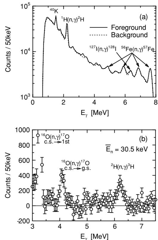
FIG. 3.  $\gamma$ -ray pulse height spectra from the  ${}^2\text{H}(n, \gamma){}^3\text{H}$  reaction. (a) Foreground and background spectra are respectively shown as the solid and dotted lines at  $10 < E_n < 80$  keV. (b) Background subtracted spectrum at  $20 < E_n < 40$  keV is shown.
