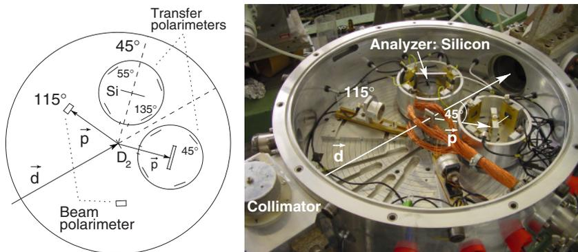
FIG. 2. (Color online) Setup in the scattering chamber: Two transfer polarimeters at  $\theta = 45^\circ$ , the beam polarimeter detectors at  $\theta = 115^\circ$  and a Cu braid around the target.
