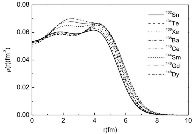
FIG. 1. Variation of charge density distributions for the  $N = 82$  isotonic nuclei calculated with the RMF model.
