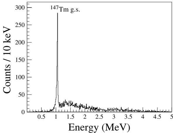
FIG. 1. Energy spectrum of decay events from the  $A = 147$  run in the  $^{58}\text{Ni} + ^{92}\text{Mo}$  reaction. The 1.051 MeV proton line is from the ground-state decay of  $^{147}\text{Tm}$ .
