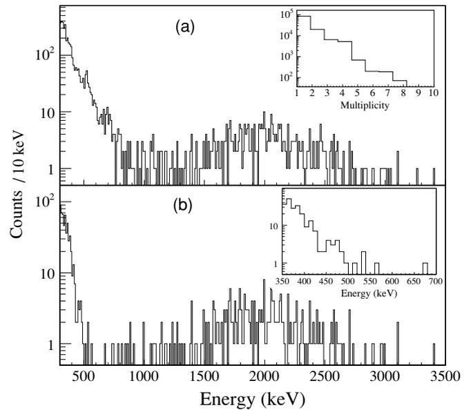
FIG. 2. (a) Energy spectrum in all strips on one side of the DSSD; the inset shows the multiplicity for  $\beta$  events below 400 keV. (b) Energy spectrum obtained with the condition of multiplicity  $M = 1$  and energy difference of less than  $3\sigma$  (05 keV) on both sides of the DSSD. The region of interest is expanded in the inset.
