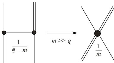
FIG. 1. The quark exchange diagram (left) in the Faddeev approach [13,14] and its static limit (right).
