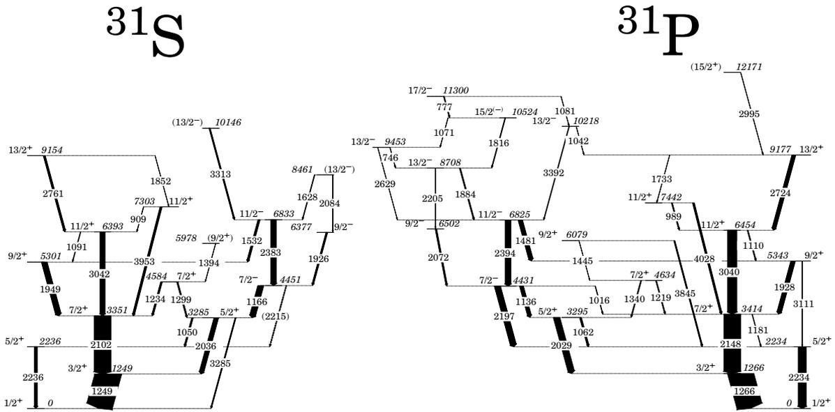
FIG. 1. Comparison of the high spin level schemes for  $^{31}\text{S}$  (left) and  $^{31}\text{P}$  (right). Transition and level energies are in keV. The width of the arrows represents the relative intensity of the transitions in each nucleus.
