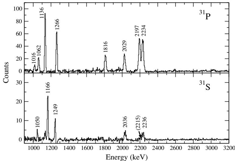
FIG. 4. The top spectrum shows transitions above the  $7/2^-$  level in  $^{31}\text{P}$  and is double-gated by the 1136- and 2029-keV transitions in the  $\gamma$ - $\gamma$ - $\gamma$  cube. The bottom spectrum contains transitions above the  $7/2^-$  level in  $^{31}\text{S}$  and is double-gated by the 1166- and 2036-keV transitions in the  $\gamma$ - $\gamma$ - $\gamma$  cube. Mirror transitions of interest are labeled with their energy in keV.
