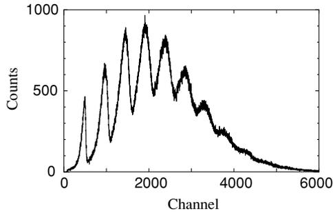
FIG. 2. Pile-up spectrum of the LCS photons measured with a large volume ( $8'' \times 12''$ ) NaI(Tl) scintillation detector. In this spectrum the average photon number per laser pulse is 5.4, which leads to the LCS photon intensity of  $1.08 \times 10^4/\text{s}$ .
