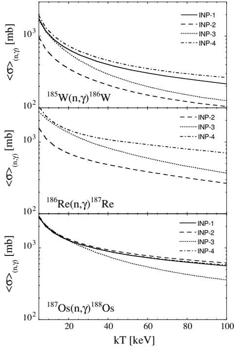
FIG. 7. Stellar Maxwellian-averaged neutron capture cross sections for  $^{185}\text{W}$  (upper panel),  $^{186}\text{Re}$  (middle panel), and  $^{187}\text{Os}$  (lower panel) calculated on the basis of the HF input defined in Table II.
