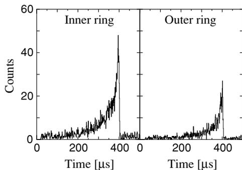
FIG. 3. Typical time-correlated spectra between laser pulses and neutrons detected in the inner and outer rings. The time correlation was measured by using a TAC module with the neutron signal and the 2-kHz laser pulse being the start and stop, respectively.
