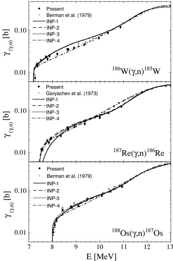
FIG. 5. Comparison between measured and calculated photoneutron cross sections for  $^{186}\text{W}(\gamma, n)^{185}\text{W}$  (upper panel),  $^{187}\text{Re}(\gamma, n)^{186}\text{Re}$  (middle panel), and  $^{188}\text{Os}(\gamma, n)^{187}\text{Os}$  (lower panel). The different theoretical predictions correspond to the input defined in Table II.
