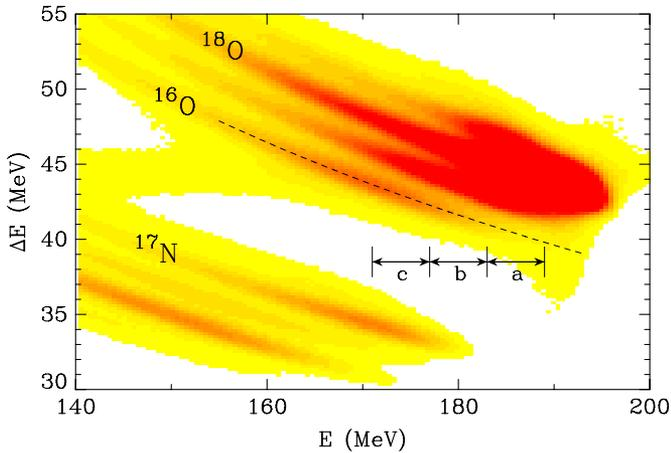
FIG. 1. (Color online)  $E$ - $\Delta E$  plot measured by a Si  $\Delta E$ - $E$  detector in the reaction of a 200-MeV  $^{18}\text{O}$  beam with a  $^{238}\text{U}$  target. Dashed line represents a calculated energy loss for  $^{16}\text{O}$  particles. See the caption of Fig. 2 for the energy ranges of  $a$ ,  $b$ , and  $c$ .
