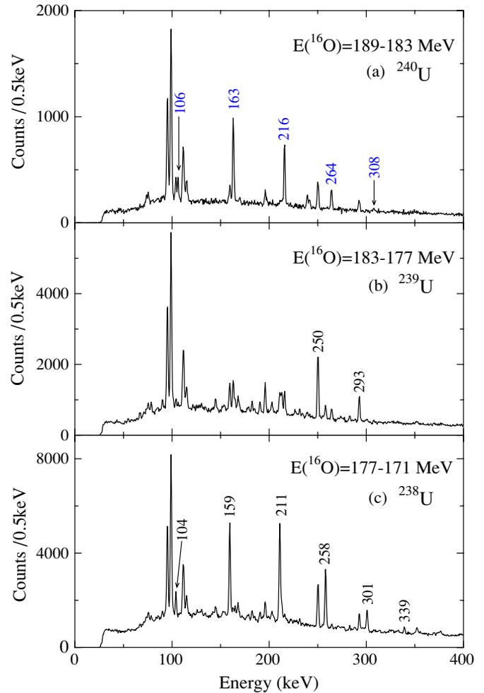
FIG. 2. (Color online)  $\gamma$ -ray spectra obtained by setting the gates on  $^{16}\text{O}$  whose total energies are (a) 189–183, (b) 183–177, and (c) 177–171 MeV, respectively. These energy ranges are depicted in Fig. 1.  $\gamma$  peaks labeled by energies in the spectra of (a), (b), and (c) are the transitions in  $^{240}\text{U}$ ,  $^{239}\text{U}$ , and  $^{238}\text{U}$ , respectively.
