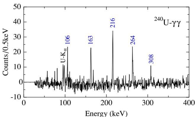
FIG. 4. (Color online)  $\gamma$ - $\gamma$  coincidence spectrum for ground-state band transitions in  $^{240}\text{U}$ , obtained by the sum of spectra in coincidence with 163-, 216-, and 264-keV  $\gamma$  rays.
