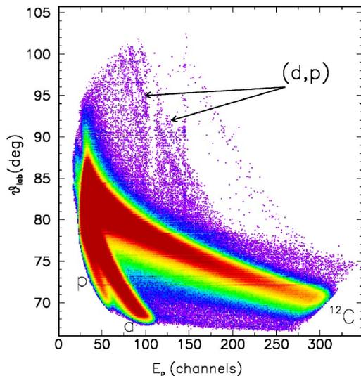
FIG. 2. (Color online) Angle of particles measured in the upstream telescope as a function of energy, without any gates imposed. Elastic scattering of carbon atoms, deuterons and protons from the target and reaction protons from the  $(d,p)$  reaction are indicated.
