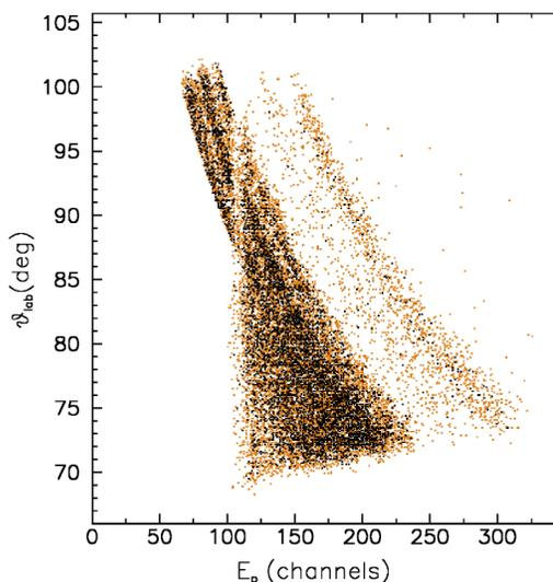
FIG. 3. (Color online) Angle of particles measured in the downstream telescope as a function of energy, with proton gates imposed. Proton identification was based on  $\Delta E$  versus  $E$  characteristics for those particles passing through the  $\Delta E$  detector and on the kinematics for the lower energy protons, i.e., those below channel 100 (see text).
