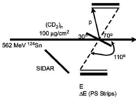
FIG. 1. Experimental setup with the  $^{124}\text{Sn}$  beam impinging on a  $100\ \mu\text{g}/\text{cm}^2$   $\text{CD}_2$  target rotated  $30^\circ$  with respect to the beam direction. Protons following a  $(d,p)$  reaction were measured in two detector telescopes that covered  $70^\circ$  to  $110^\circ$  in the laboratory and in SIDAR that covered  $130^\circ$  to  $160^\circ$ .
