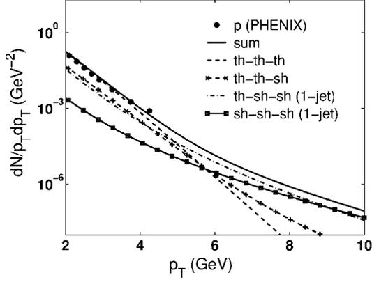
FIG. 5. Transverse momentum distribution of proton in Au-Au collisions. Data are from Ref. [16]. The solid line is the sum of four contributions to the recombination of partons:  $TTT$  (dashed line);  $TTS$  (line with crosses);  $TTS$ , one thermal parton with two shower partons in one jet (dashed-dot line); and  $SSS$ , three shower partons from one jet (line with squares).
