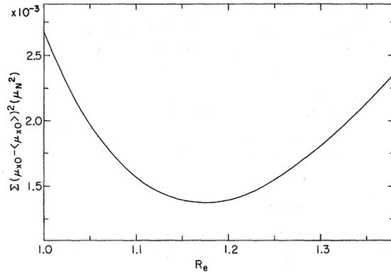
FIG. 2.  $\sum (\mu_{x0} - \langle \mu_{x0} \rangle)^2$  versus  $R_e$  from approach No. 2.
