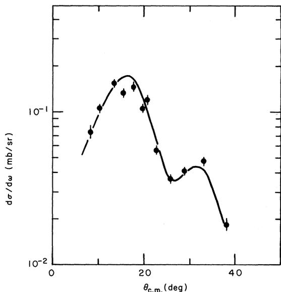
FIG. 2. Angular distribution of the deuterons leading to the ground state in the  $^{94}\text{Zr}(^3\text{He}, d)^{95}\text{Nb}$  reaction. The solid line is the DWBA calculation for an  $l=4$  transfer.
