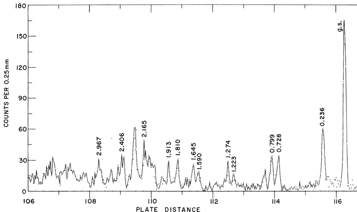
FIG. 1. Typical deuteron spectrum from the  $^{94}\text{Zr}(^3\text{He}, d)^{95}\text{Nb}$  reaction at  $\theta_{\text{lab}} = 19^\circ$ .
