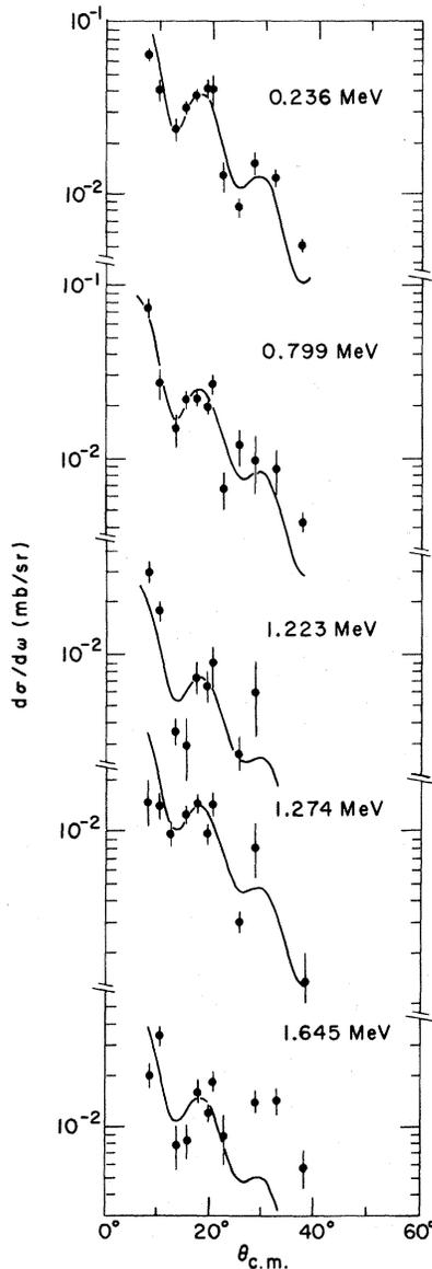
FIG. 3. Angular distributions for five levels excited by  $l=1$  transfer in the  $^{94}\text{Zr}(^3\text{He}, d)^{95}\text{Nb}$  reaction. The solid curves are results of the DWBA calculations.
