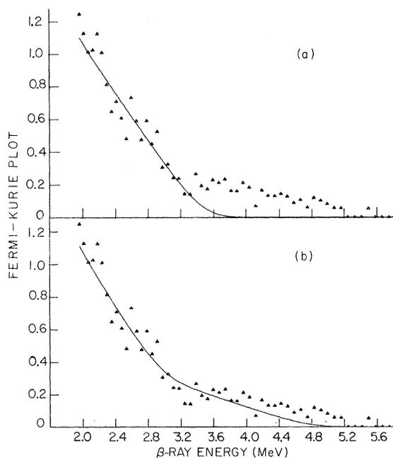
FIG. 4. (a) Fermi plot of the  $\beta$ -ray spectrum in coincidence with the 0.603-MeV transition in the decay of  $^{91}\text{Rb}$  and the fit obtained with 5.8%  $\beta$  branching to the 1.041-MeV level of  $^{91}\text{Sr}$ . (b) Fermi plot of the  $\beta$ -ray spectrum in coincidence with the 0.603-MeV transition in the decay of  $^{91}\text{Rb}$  and the fit obtained with 0.6%  $\beta$  branching to the 1.041-MeV level of  $^{91}\text{Sr}$ .
