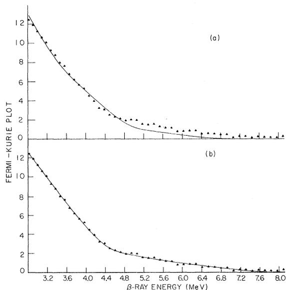
FIG. 5. (a) Fermi plot of the  $\beta$  singles spectrum for the decay of  $^{92}\text{Kr}$  and the fit obtained with 50%  $\beta$  branching to the ground state of  $^{92}\text{Rb}$ . (b) Fermi plot of the  $\beta$  singles spectrum for the decay of  $^{92}\text{Kr}$  and the fit obtained with 2%  $\beta$  branching to the ground state of  $^{92}\text{Rb}$ .
