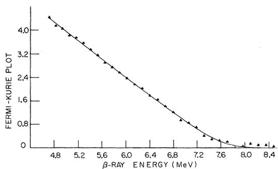
FIG. 6. Fermi plot of the  $\beta$  singles spectrum for the decay of  $^{92}\text{Rb}$ .
