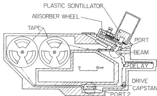
FIG. 1. Moving tape collector.
