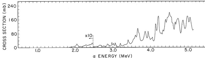
FIG. 2. These data were obtained by means of a "drive-in" target made by bombarding a tantalum blank with 25-keV  $^{22}\text{Ne}$  ions in a magnetic separator. The target thickness is  $\sim 24$  keV for 2-MeV  $\alpha$  particles. The cross-section scale has been obtained by normalizing to the gas target data.
