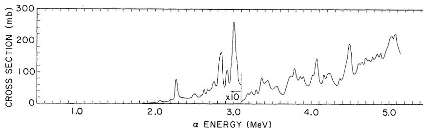
FIG. 1. These data were obtained by means of a "drive-in" target made by bombarding a tantalum blank with 25-keV  $^{21}\text{Ne}$  ions in a magnetic separator. The target thickness is  $\sim 24$  keV at 2 MeV. The cross-section scale has been obtained by normalizing to the gas target data.
