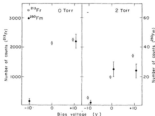
FIG. 3. The dependence of the recoil yield on the bias voltage applied between the wheel and the detectors and on the pressure of Ar gas introduced into the space between the detector faces and the rim of the wheel. Open circles refer to  $^{213}\text{Fr}$  from EC of  $^{213}\text{Ra}$ , and the black circles to  $^{250}\text{Fm}$  from  $^{250\text{m}}\text{Fm}$ .
