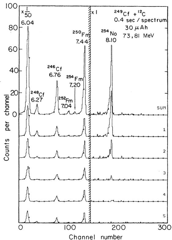
FIG. 5. The  $\alpha$ -particle spectra resulting from the same bombardments as those in Fig. 3 but recorded by the detectors in the off-wheel position.
