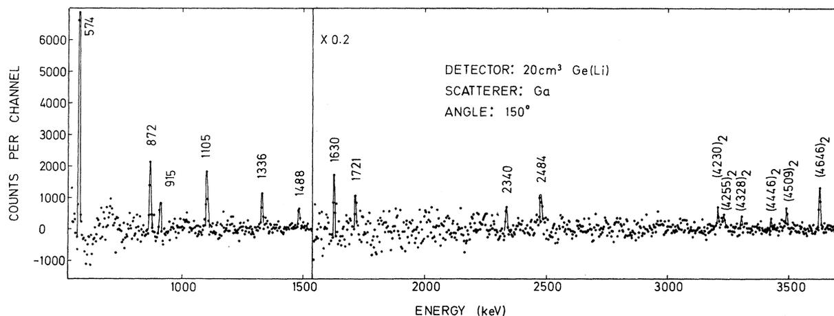
FIG. 2. Low-energy part of the scattered spectrum, from a  $3\text{-g/cm}^2$  Ga target, obtained after an artificial subtraction of an exponential "background." The  $\gamma$  source was obtained from the  $\text{Cu}(n,\gamma)$  reaction. A  $20\text{-cm}^3$  detector was used at a scattering angle of  $150^\circ$ .  $\gamma$  lines denoted by a subscript 2 refer to double-escape peaks; other lines refer to photopeaks.
