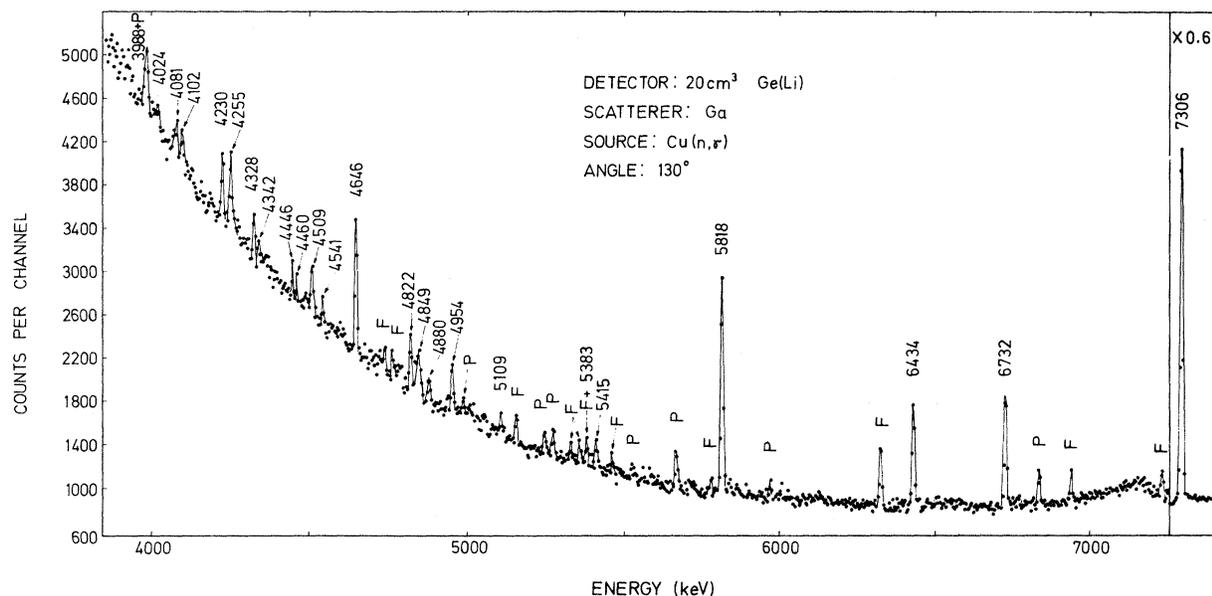
FIG. 1. High-energy part of the scattered  $\gamma$  spectrum from a Ga target at an angle of  $140^\circ$  measured by a  $20\text{-cm}^3$  Ge(Li) detector. The  $\gamma$  source was obtained from the  $\text{Cu}(n,\gamma)$  reaction.  $\gamma$  lines denoted by P and F refer to photopeaks and first-escape peaks, respectively; other lines refer to double-escape peaks.
