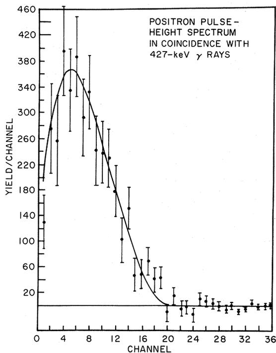
FIG. 5. Spectrum of positrons in coincidence with 426.9-keV  $\gamma$  rays. The curve represents the spectral shape deduced for a positron end-point energy of 2.96 MeV.
