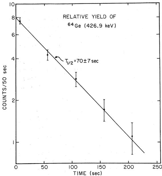
FIG. 3. Relative yield of the 426.9-keV transition as a function of time. The straight line represents the nonlinear least-squares fit for a half-life of 70 sec. The yield has been corrected for a small contribution from  $^{66}\text{Ge}$ .
