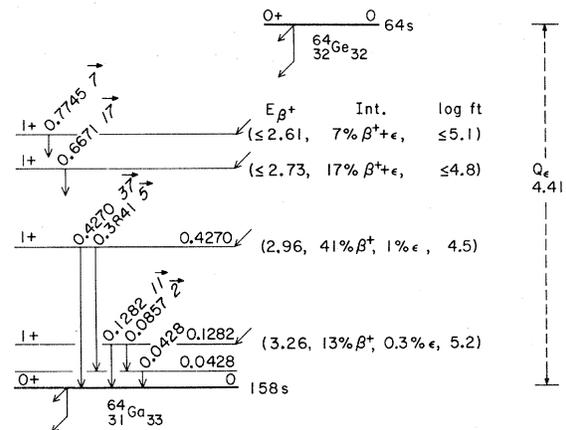
FIG. 4. Decay scheme of  $^{64}\text{Ge}$ , taken mainly from RA. The  $\beta^+$ -ray energies and  $\log ft$  values have been recomputed, using the present measured mass. The average of the present half-life and that of RA is  $64.4 \pm 2.4$  sec. The half-life shown for  $^{64}\text{Ga}$  is an average of the present value and that of Ref. 14. All energies are in MeV.
