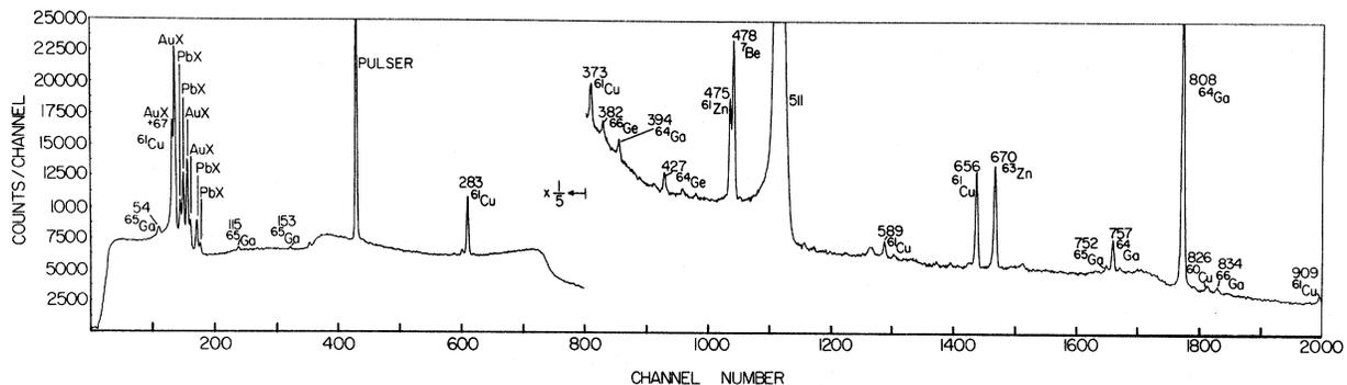
FIG. 2. Part of the  $\gamma$  spectrum for first 50-sec time bin. The 478-keV peak appeared even in the absence of the rabbit, and is attributed to  $^7\text{Be}$  contamination of the Pb shielding blocks surrounding the detectors.  $\gamma$ -ray energies are given to the nearest keV.
