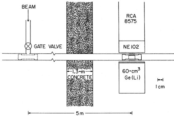
FIG. 1. Experimental configuration for off-line positron- $\gamma$  coincidence measurement. Not shown are Pb shielding blocks surrounding both detectors.
