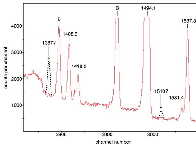
FIG. 6. (Color online) Evidence from the  $\gamma$ -ray singles data that lines adopted [2] at 1387 and 1510 keV are spurious; dashed lines indicate the reported intensities of these transitions. The spectrum also shows the strongest coincidence sum peak (at 1397.6 1397.6 =  $\Sigma 123 + 1274$  keV) in the spectrum and the strong room background peak (at 1460.8 keV) from  $^{40}\text{K}$ .
