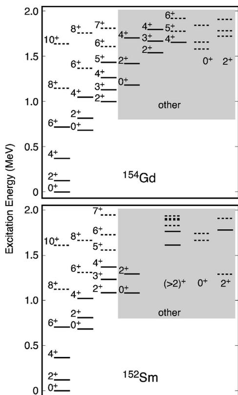
FIG. 10. Comparison of the low-lying positive-parity states in  $^{152}\text{Sm}$  (bold lines indicate states populated in the decay of  $^{152}\text{gEu}$  and dashed lines indicate levels observed through other methods of spectroscopy; data from [1]) and  $^{154}\text{Gd}$  (bold lines from the present work and dashed lines from [2]), cf. Fig. 1.
