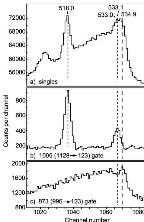
FIG. 11. The weak 533 keV ( $1661 \rightarrow 1128$ ) and 535 keV ( $1531 \rightarrow 996$ ) transitions coincide with a Compton artifact in (a) the  $\gamma$ -ray singles spectrum, but are measured through (b) the 1005 keV and (c) the 873 keV coincidence spectra.
