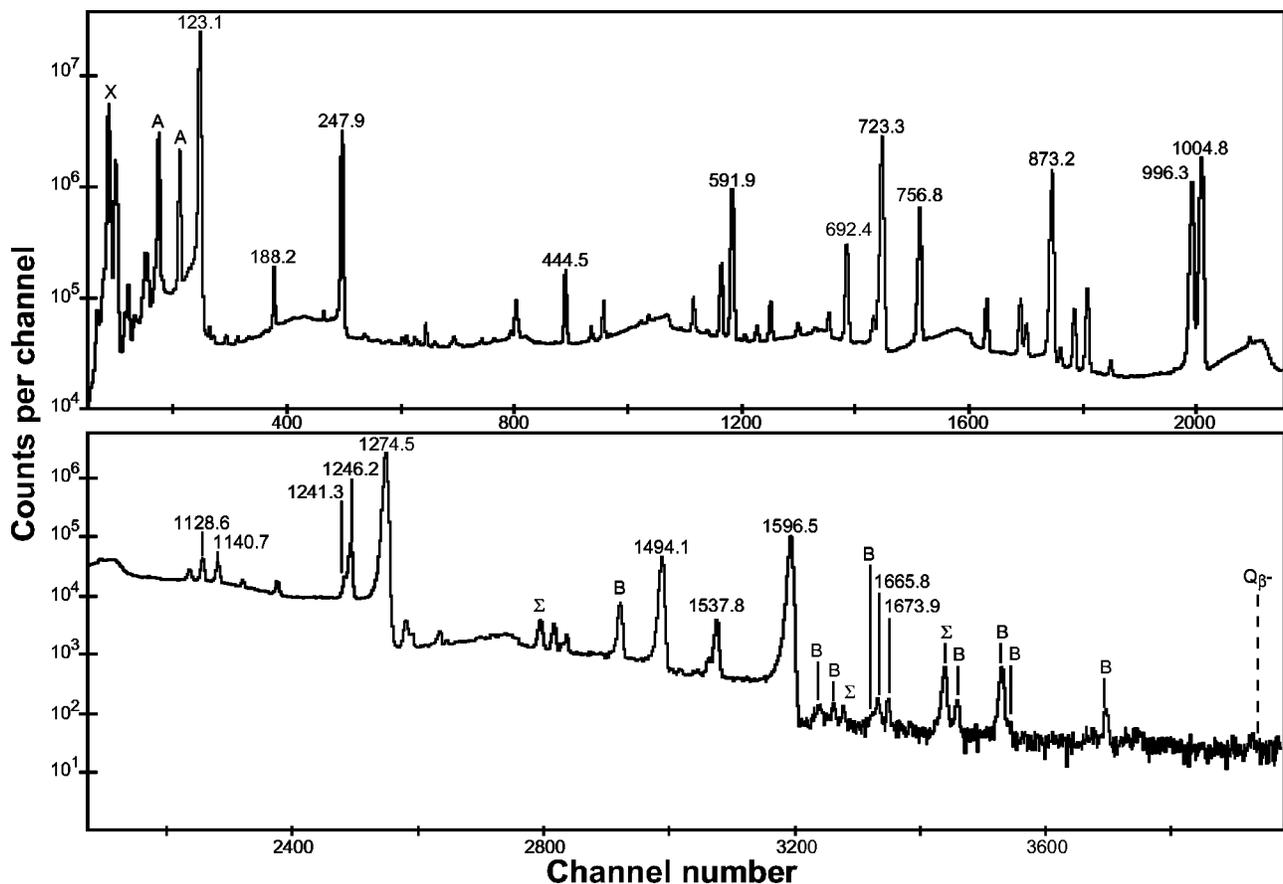
FIG. 2. The singles  $\gamma$ -ray spectrum for  $^{154}\text{Eu}$  decay obtained in the present study. Peaks marked X are x rays; A are the strong lines from the decay of  $^{155}\text{Eu}$  at 86 and 105 keV;  $\Sigma$  are from coincidence summing; and B are from room background. Energies of selected lines are given in keV, and  $Q_{\beta^-}=1968.5$  keV is indicated.
