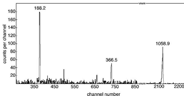
FIG. 5. The coincident  $\gamma$ -ray spectrum associated with the 349 keV ( $1531 \rightarrow 1182$ ) transition. This establishes for the first time that the  $0^+$  1182 keV level is populated (indirectly) in the decay of  $^{154}\text{Eu}$ .
