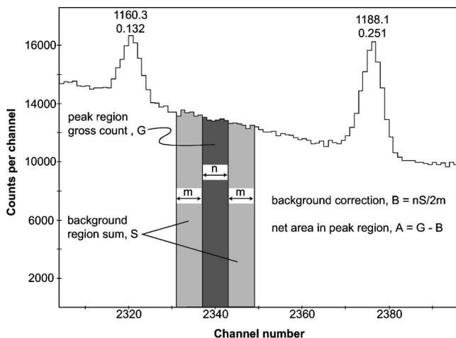
FIG. 4. An illustration of the data used to establish an upper intensity limit for a  $\gamma$ -ray line by use of the method of Currie [13]. This figure is discussed further in the text.
