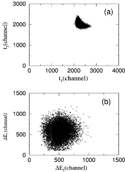
FIG. 1. The (a) time and (b) energy loss correlations of simultaneously detected fission fragments at  $E_{cm}=85.3$  MeV.
