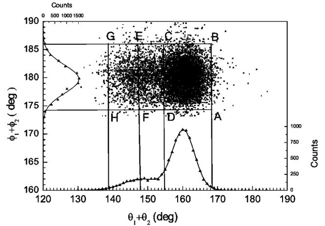
FIG. 2. Distributions of complimentary fission fragments in  $(\theta, \phi)$  at  $E_{cm}=85.3$  MeV. Rectangle ABCD indicates the gate used to select the fusion-fission events for mass determination. Rectangles ABEF and ABGH indicate the gate used to add 50% and 100% of TF events, respectively.
