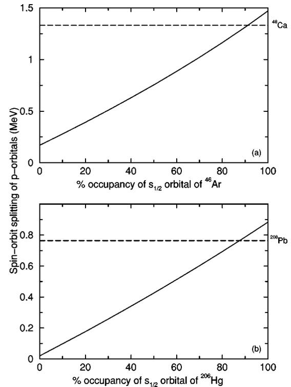
FIG. 5. Spin-orbit splittings of the  $p$  orbitals (in MeV) for  $^{46}\text{Ar}$  and  $^{206}\text{Hg}$  as a function of the occupancy of the  $s_{1/2}$  proton orbital. The dashed lines show spin-orbit splittings for the two doubly magic nuclei  $^{48}\text{Ca}$  and  $^{208}\text{Pb}$ , respectively.
