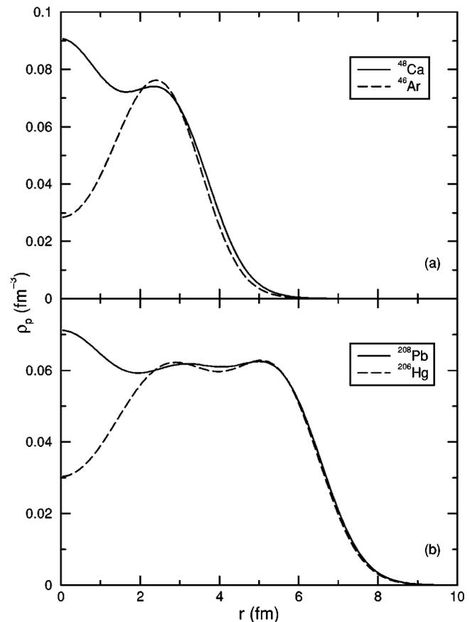
FIG. 1. Proton (point) densities for (a)  $^{46}\text{Ar}$  and  $^{48}\text{Ca}$  and for (b)  $^{206}\text{Hg}$  and  $^{208}\text{Pb}$  computed using the relativistic parametrization of Ref. [24]. The development of a “proton hole” in the interior of the nucleus is readily observed.
