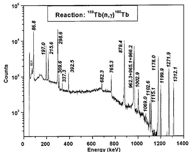
FIG. 1.  $\gamma$  Ray energy spectrum of the irradiated  $Tb_4O_7$  sample.
