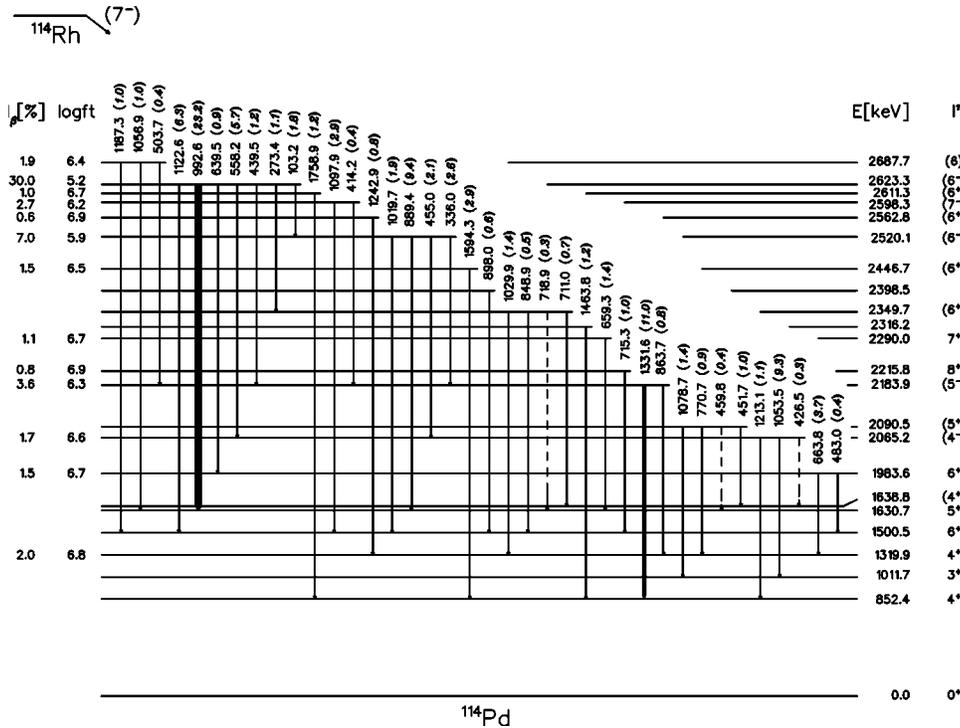
FIG. 4. Decay scheme of the higher-spin level of  $^{114}\text{Rh}$  (continued). Levels and transitions belonging to the band on the 1639 keV level are also shown in Fig. 3.
