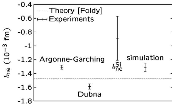
FIG. 2. Comparison of the theoretical  $b_{\text{ne}}$  value (3) with the Argonne-Garching and Dubna experimental values and with the result (12). The simulated point has the Argonne-Garching value with an error bar of  $0.06\times 10^{-3}$  fm, as estimated in the text.
