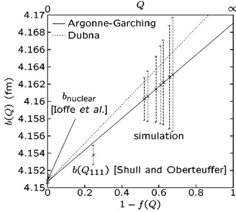
FIG. 1. Experimental  $b_{\text{nuclear}}$  of Eq. (11) and  $b(Q_{111})$  of Eq. (10) compared with the theoretical curves (4) for  $b_{\text{nuclear}}=4.1507$  fm,  $b_{\text{ne}}=-1.31$  (Argonne-Garching), and  $-1.59\times 10^{-3}$  fm (Dubna). The simulated points correspond to the reflections of Table I; they are calculated with the Argonne-Garching  $b_{\text{ne}}$  value, with error bars only due to the uncertainty on the temperature factor (9).
