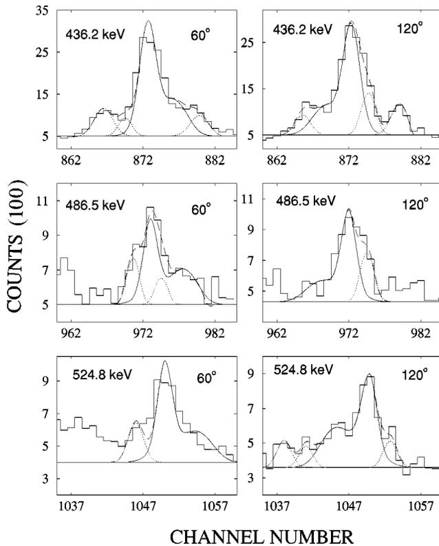
FIG. 3. Experimental and theoretical line shapes for the 436, 486, and 525 keV  $\gamma$  rays at the forward  $60^\circ$  and backward  $120^\circ$  angles with respect to the beam direction in the  $B3$  band of  $^{136}\text{Ce}$ . The contaminant peaks are shown in dotted lines and lineshapes for  $\gamma$  rays of interest are shown with solid lines.
