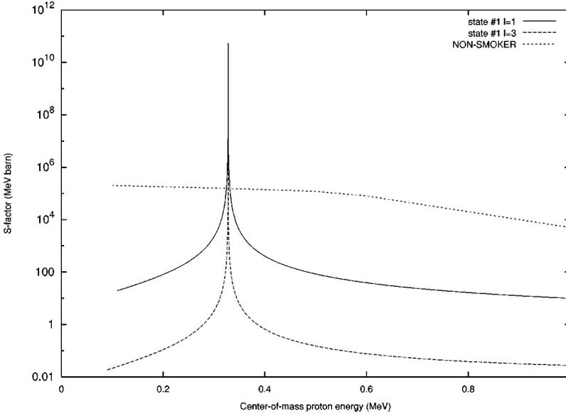
FIG. 1. Astrophysical  $S$  factor calculated using the single resonance formula as a function of proton center-of-mass energy for the resonance in  $^{46}\text{Cr}$  corresponding to the first  $^{46}\text{Ti}$  level in Table II. The results of the statistical code NON-SMOKER are included for comparison.
