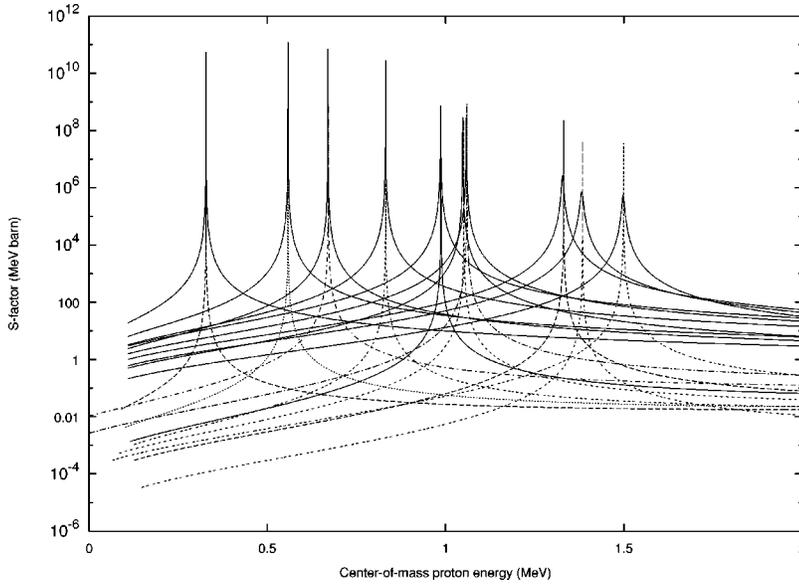
FIG. 2. Astrophysical  $S$  factor calculated using the single resonance formula as a function of proton's center-of-mass energy for the resonances in  $^{46}\text{Cr}$  corresponding to all ten  $^{46}\text{Ti}$  levels in Table II.
