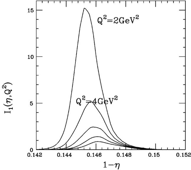
FIG. 3. Important region of integration for  $F_1$ , Eq. (30). The curves show the derivative of  $I_1$  for values of  $Q^2 = 2, 4, 6, 8, 10$   $\text{GeV}^2$ , with the larger values occurring for the smaller values of  $Q^2$ .
