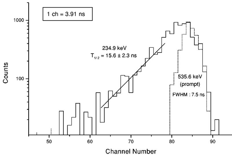
FIG. 1. Typical beam- $\gamma$ -time spectra corresponding to 234.9 keV (delayed) and 535.6 keV (prompt) gates.
